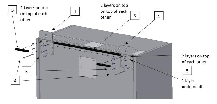
Tighten screw 4 with max. 2 Nm or screw 3 with max. 2.5 Nm!
